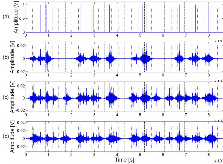
**Figure 11.** The interference to User 2 by close users, (a) TH-PPM signals, (b) the response with the interference from one user with distance of 30 cm, (c) the response with the interferences from two users with distances of 30 cm and 15 cm, and (d) the response with the interference from three users with distances of 30 cm, 15 cm and 7.5 cm.
