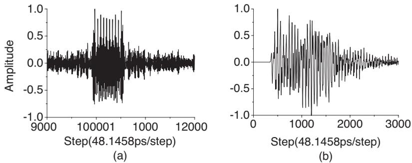
**Figure 6.** The normalized response of waveform strings with periodicity of 60 time steps; (a) for TR waveform, and (b) for Gaussian pulse.
