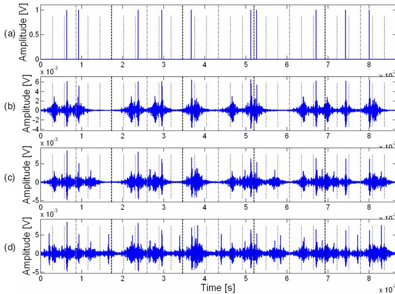
**Figure 12.** The interference to User 3 by close users, (a) TH-PPM signals, (b) the response with the interference from one user with distance of 30 cm, (c) the response with the interferences from two users with distances of 30 cm and 15 cm, and (d) the response with the interference from three users with distances of 30 cm, 15 cm and 7.5 cm.
