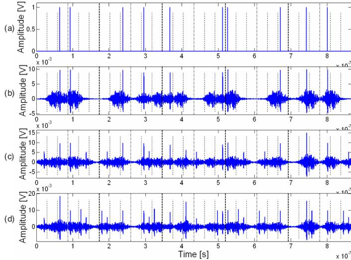
**Figure 10.** The interference to User 1 by close users, (a) TH-PPM signals, (b) the response with the interference from one user with distance of 30 cm, (c) the response with the interferences from two users with distances of 30 cm and 15 cm, and (d) the response with the interference from three users with distances of 30 cm, 15 cm and 7.5 cm.
