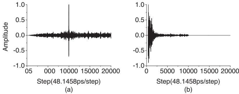
**Figure 2.** The normalized single pulse response between Antenna 0 and Antenna 1; (a) channel response of time reversal waveform and (b) channel response of Gaussian pulse.
