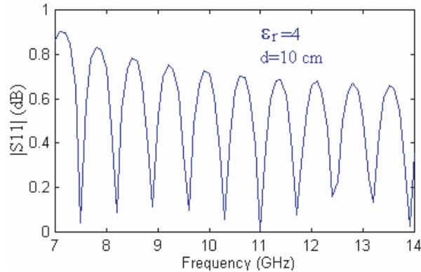
**Figure 5.** Frequency response of the reflection coefficient of the waveguide system.
