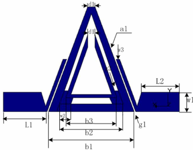
**Figure 2.** Configuration of the dual-mode dual-band bandpass filter.
