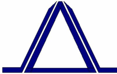
**Figure 1.** Configuration of the conventional triangular dual-mode filter.
