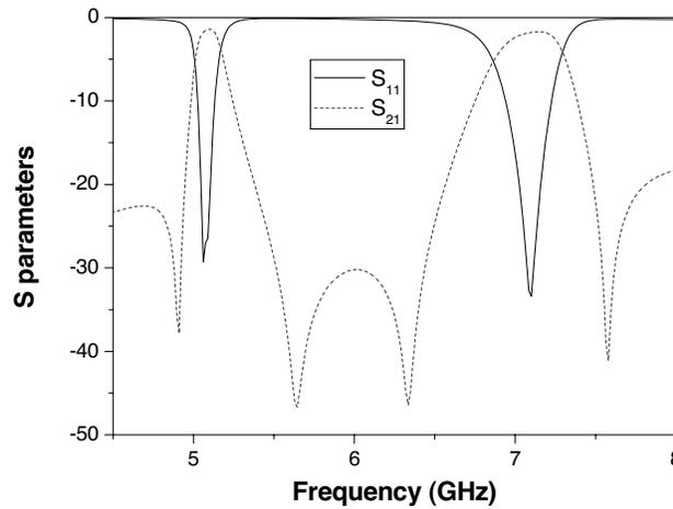
**Figure 3.** Simulation results of proposed dual-band filter.
