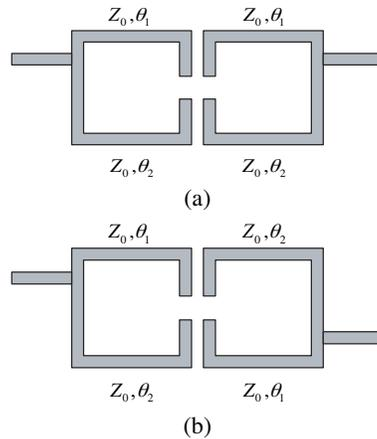
**Figure 1.** (a) Non-0° feed structure. (b) 0° feed structure.
