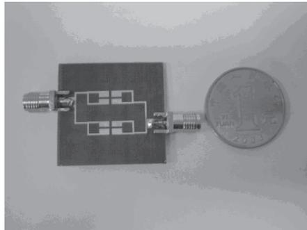
**Figure 4.** Photograph of the fabricated dual-band filter.
