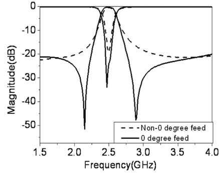
**Figure 2.** Simulated results with non-0° and 0° feed structures.
