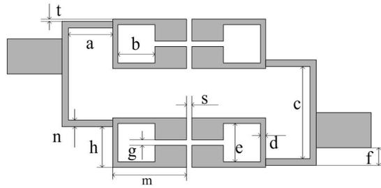
**Figure 3.** Layout of the proposed dual-band filter. Dimensions:  $a = 3.3$  mm,  $b = e = 3$  mm,  $c = 8.5$  mm,  $d = 0.5$  mm,  $f = 1.5$  mm,  $g = 0.6$  mm,  $h = 3.4$  mm,  $m = 6.5$  mm,  $n = 0.5$  mm,  $s = 0.7$  mm,  $t = 0.1$  mm.
