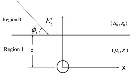
**Figure 1.** Geometry of buried PECM cylinder inside a dielectric half space.
