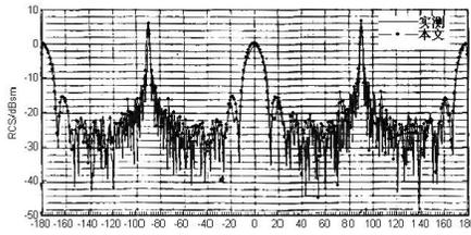
**Figure 8.** The RCS of the cylindrical above.
