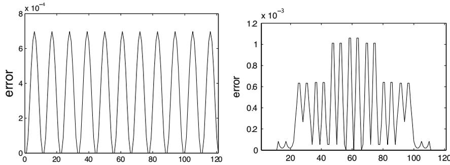
**Figure 2.** The relative errors of **Figure 3.** the radius of a cylindrical surface. the radius of a spherical surface.
