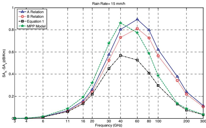
**Figure 4.** The difference between horizontal specific attenuation and vertical specific attenuation vs. frequency.
