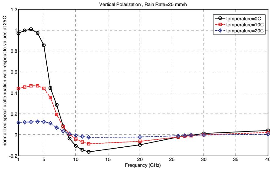
**Figure 7.** Normalized vertical specific attenuation of realistic raindrops with respect to specific attenuation values at  $25^{\circ}$ C.
