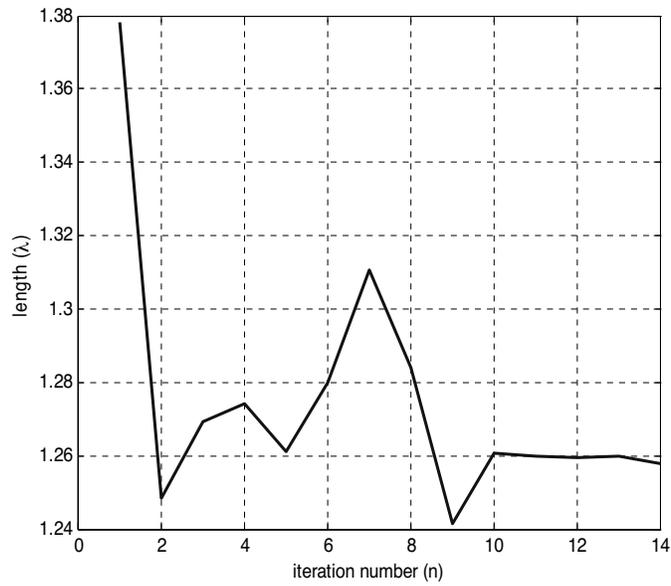
**Figure 3.** Length of dipole versus IWO iteration number.
