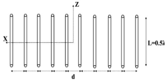
**Figure 4.** Linear array of 10 half-wavelength dipoles [13].
