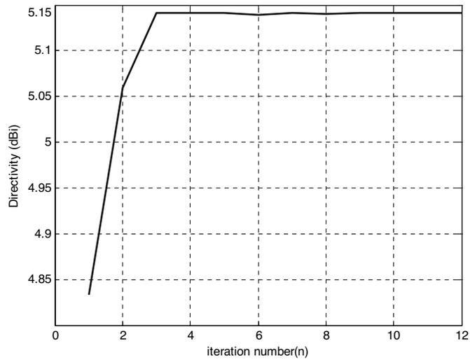
**Figure 2.** Directivity of dipole versus IWO iteration number.
