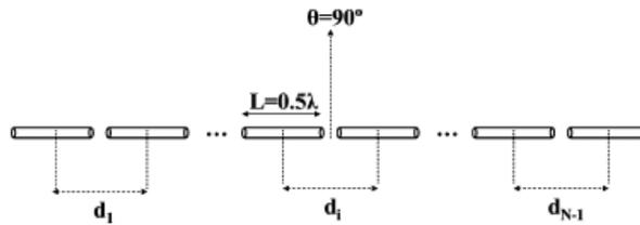
**Figure 10.** Collinear array of  $N$  half-wavelength dipoles [13].
