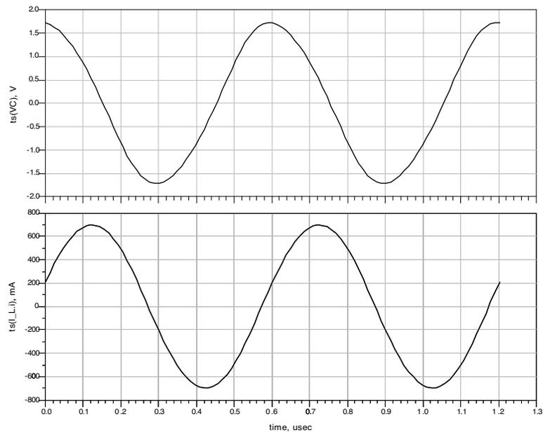
**Figure 3.** Steady state response of diode oscillator.
