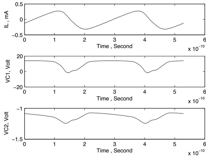
**Figure 7.** Steady state response of Colpitz oscillator.
