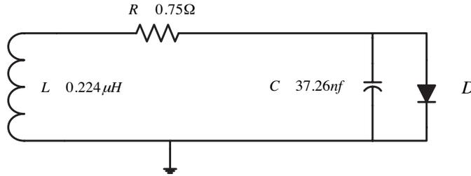
**Figure 2.** Diode oscillator.
