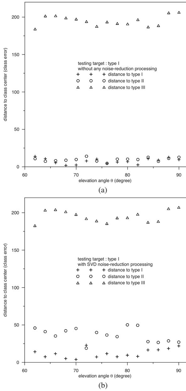
**Figure 4.** The distance (i.e., class error) to feature centers for the three known classes of ship RCS at different elevation angles  $\theta$  by using ship of type I as the testing target: (a) without any noise-reduction processing, and (b) with SVD noise-reduction processing.
