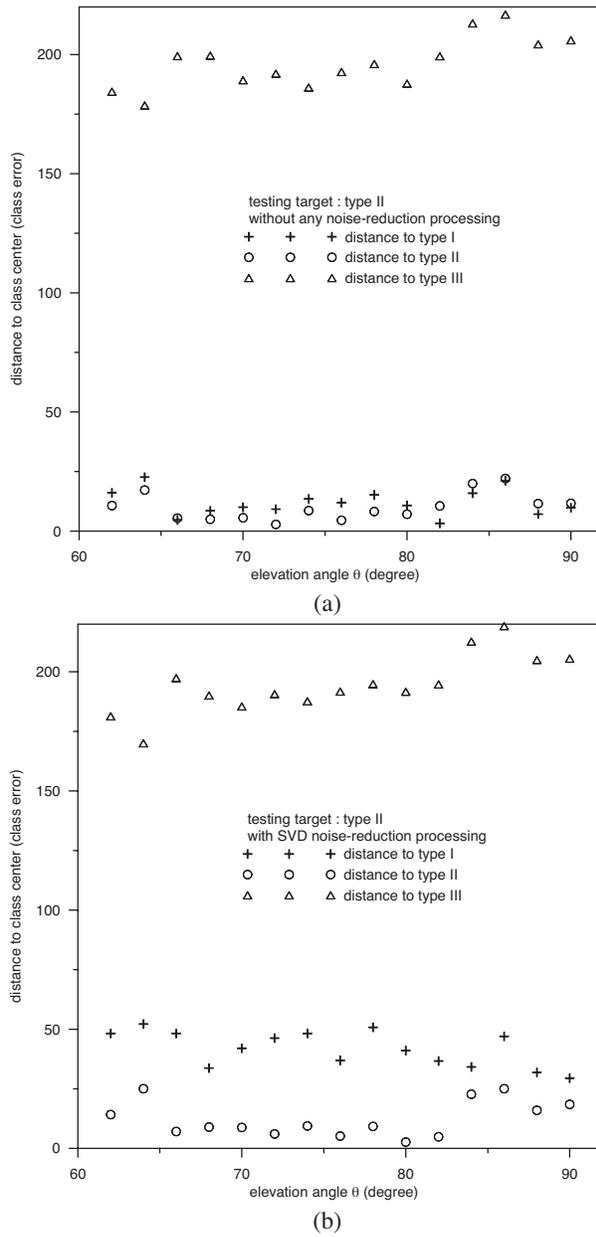
**Figure 5.** The distance (i.e., class error) to feature centers for the three known classes of ship RCS at different elevation angles  $\theta$  by using ship of type II as the testing target: (a) without any noise-reduction processing, and (b) with SVD noise-reduction processing.
