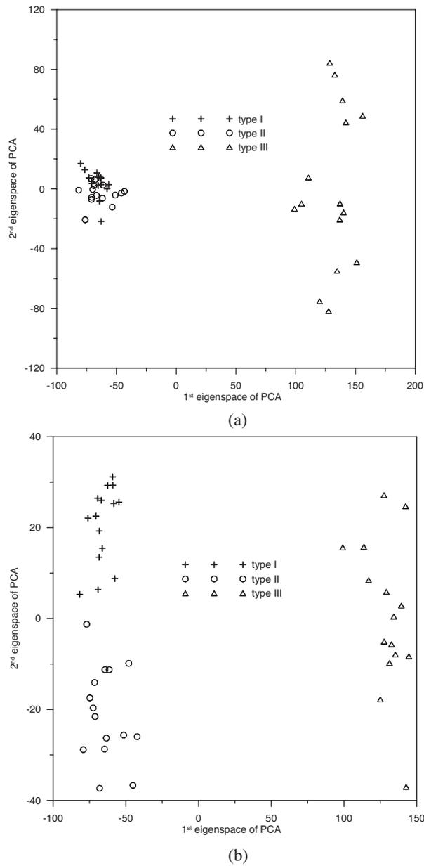
**Figure 3.** The projected features on the 2-dimensional PCA space for the training RCS data of the three known ships: (a) without any noise-reduction processing, and (b) with SVD noise-reduction processing.
