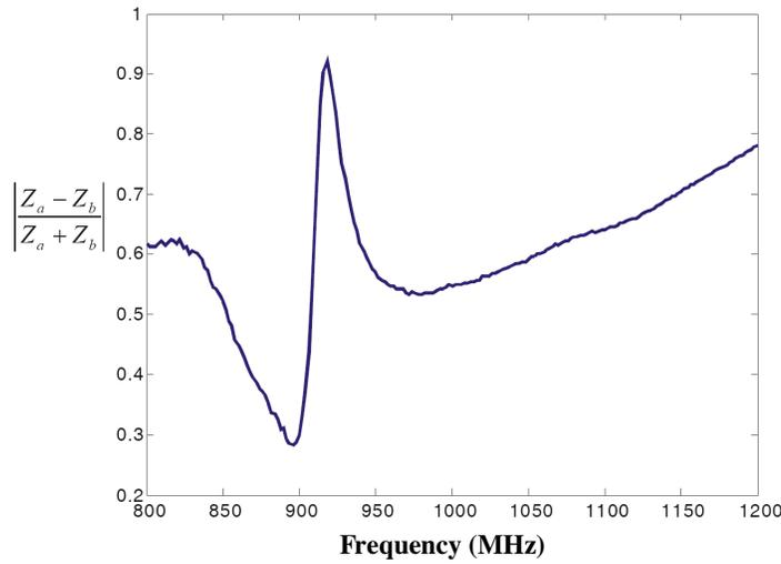
**Figure 11.** Evaluation of unbalance of the patch antenna.
