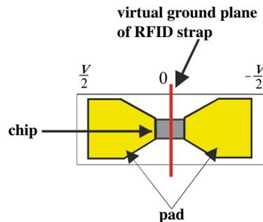
**Figure 1.** An RFID trap and its virtual ground surface.
