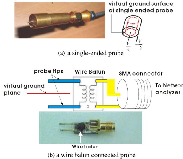
**Figure 2.** Existing method for RFID tag antenna measurement.
