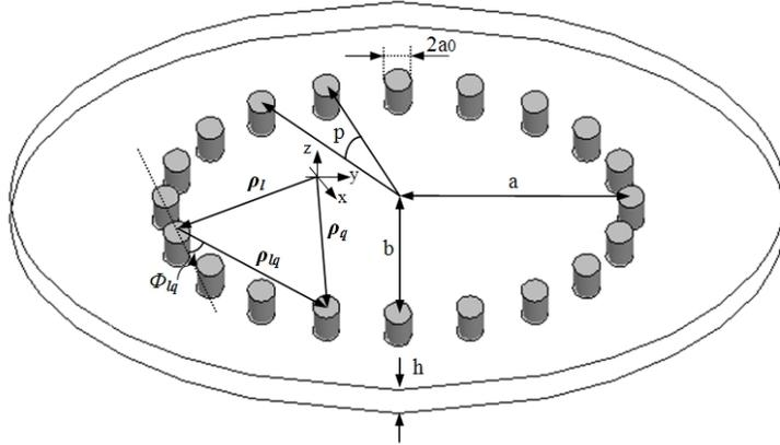
**Figure 1.** An elliptic SIW resonator, where in particular the angular pitch  $p$ , the via hole radius  $a_0$ , the semi major axis  $a$ , the semi minor axis  $b$  and the dielectric substrate height  $h$  are shown.
