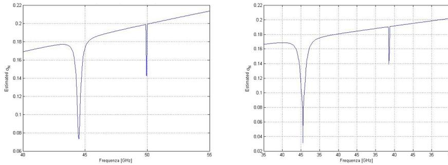
**Figure 2.** The estimated  $\sigma_N$  as a function of the real frequency for two SIW elliptical resonators. (left:  $a = 3.125$  mm,  $b = 2.500$  mm; right:  $a = 3.800$  mm,  $b = 3.040$  mm;  $\epsilon_r = 2.2$ ).
