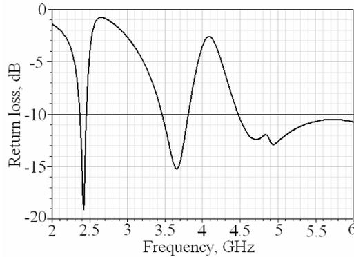
**Figure 3.** Return loss changes with frequency for proposed antenna with the parameters.  $r_1 = 4.1$  mm,  $r_2 = 7.75$  mm,  $t = 0.4$  mm,  $w = 1.1$  mm,  $s = 1$  mm,  $h = 0.4$  mm,  $w_f = 1$  mm,  $g = 0.13$  mm,  $a = 15$  mm,  $b = 10$  mm, and  $H = 0.8$  mm.
