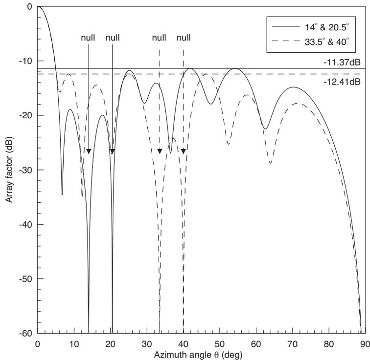
**Figure 6.** The final optimum pattern of 20-element array with the constraint of bidirectional null steering.
