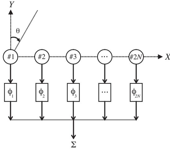
**Figure 1.** Schematic of a  $2N$ -element linear array.
