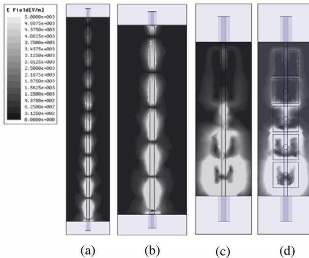
**Figure 4.** Magnitude of electrical field on the top surface of (a) 9-cell DGS filter (b) 5-cell DGS filter (c) 5-cell mushroom-like EBG filter (d) 5-cell mushroom-like EBG filter on the EBG plane. The scaling factors for (a)–(d) are not the same.  $f = (12 \text{ GHz})$ .
