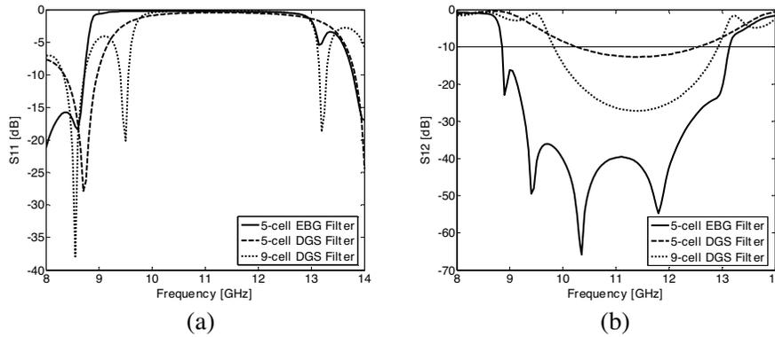
**Figure 3.** (a)  $S_{11}$  and (b)  $S_{12}$  parameters of the 1-D 5-cell mushroom-like EBG filter in comparison with 5-cell and 9-cell DGS filters.
