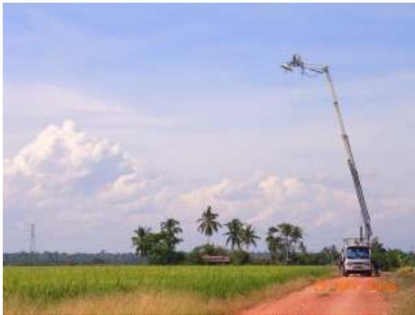
**Figure 1.** Ground-based C-band scatterometer during measurement trip.
