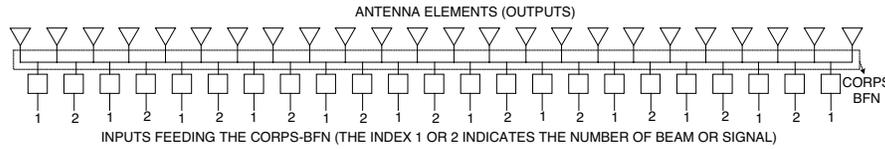
**Figure 4.** System of 24 radiators and 23 input ports with 12 complex inputs to control 24 antennas (beam # 1) and 11 complex inputs to control 22 antennas (beam # 2).
