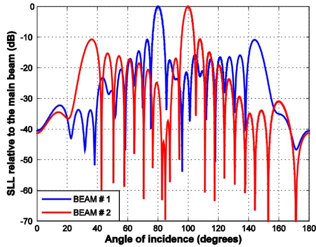
**Figure 7.** Array factor generated by the configuration 2 shown in the Fig. 4 (the direction of maximum radiation is set in  $\theta_0 = 80^\circ$  for the beam # 1 and  $\theta_0 = 100^\circ$  for the beam # 2).
