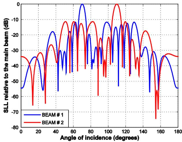
**Figure 8.** Array factor generated by the configuration 3 illustrated in the Fig. 5 (the direction of maximum radiation is set in  $\theta_0 = 70^\circ$  for the beam # 1 and  $\theta_0 = 110^\circ$  for the beam # 2).
