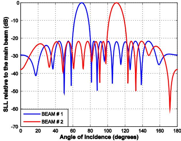
**Figure 6.** Array factor generated by the configuration 1 illustrated in the Fig. 3 (the direction of maximum radiation is set in  $\theta_0 = 70^\circ$  for the beam # 1 and  $\theta_0 = 110^\circ$  for the beam # 2).
