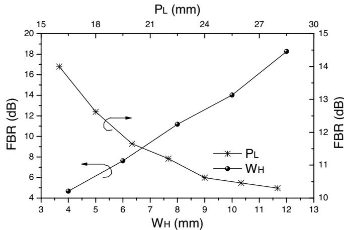
**Figure 6.** Simulated FBR of the proposed antenna versus  $W_H$  and  $P_L$ . For  $W_H$  studies:  $S_L = 14$ ,  $S_W = 1$ ,  $V_W = 0.25$ ,  $V_L = 13.5$ ,  $P_L = 25$ ,  $P_W = 19$ ,  $C_{HL} = 3$  mm,  $C_{HW} = 5$ ,  $C_{VW} = 2$ ,  $G_W = G_L = 50$ ,  $W_W = 14$ ,  $W_L = 15$  (in millimeter). For  $P_L$  studies:  $P_W = 16$ ,  $W_H = 8$ , and the others are same to those of the former.
