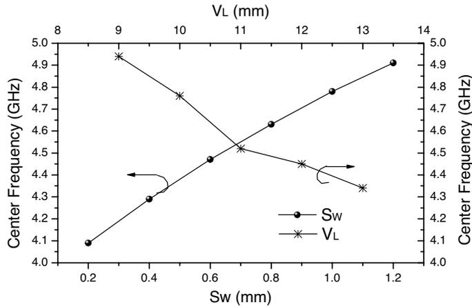
**Figure 5.** Simulated center frequency of the proposed antenna versus  $S_W$  and  $V_L$ . For  $V_L$  studies:  $S_L = 14$ ,  $S_W = 0.4$ ,  $V_W = 0.25$ ,  $P_L = 25$ ,  $P_W = 19$ ,  $C_{HL} = 3$ ,  $C_{HW} = 5$ ,  $C_{VW} = 2$ ,  $W_H = 8$ ,  $G_W = G_L = 50$ ,  $W_W = 14$ ,  $W_L = 15$  (in millimeter). For  $S_W$  studies, the other parameters are same to those in Fig. 4 ( $V_L = 13.5$ ).
