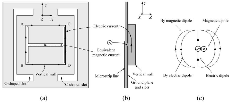
**Figure 2.** The proposed antenna is equivalent to the combination of a magnetic dipole and two electric dipoles, (a) Top view, (b) Side view, (c) Combination of a magnetic dipole and an electric dipole.
