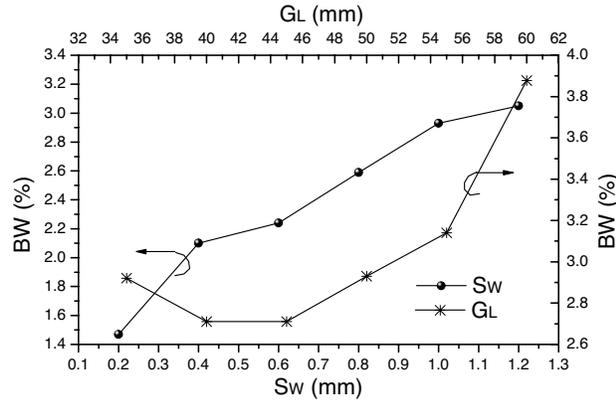
**Figure 4.** Simulated BW of the proposed antenna versus  $S_w$  and  $G_L$ . For  $S_w$  studies:  $S_L = 14$ ,  $V_W = 0.25$ ,  $V_L = 13.5$ ,  $P_L = 28$ ,  $P_W = 16$ ,  $C_{HL} = 3$ ,  $C_{HW} = 5$ ,  $C_{VW} = 2$ ,  $W_H = 8$ ,  $G_W = 50$ ,  $G_L = 50$ ,  $W_W = 14$ ,  $W_L = 15$  (in millimeter). For  $G_L$  studies:  $S_w = 1$ , and the others are same to those of the former.
