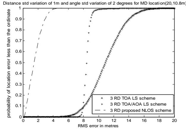
**Figure 7.** Comparison of the CDF performance using distance standard deviation  $\sigma_d = 1$  m and AOA standard deviation  $\sigma_\alpha = 2^\circ$  for *MD* located at (20 m, 10.8 m). Case B — Two *RDs* are in LOS with *MD*.
