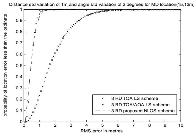
**Figure 6.** Comparison of the CDF performance using distance standard deviation  $\sigma_d = 1$  m and AOA standard deviation  $\sigma_\alpha = 2^\circ$  for  $MD$  located at (15 m, 13 m). Case A — All  $RDs$  are in LOS with  $MD$ .
