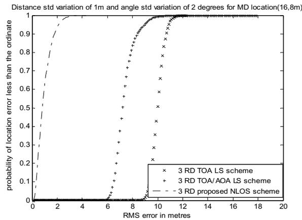
**Figure 8.** Comparison of the CDF performance using distance standard deviation  $\sigma_d = 1$  m and AOA standard deviation  $\sigma_\alpha = 2^\circ$  for *MD* located at (16 m, 8 m). Case C — One *RD* is in LOS with *MD*.
