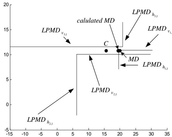
**Figure 3.** Plot of LPMDs for all the  $RDs$  for  $MD$  at (20 m, 10.8 m) at Nanyang Technological University, School of EEE, Block S1, Level 3 (S1-B3). The TOA standard deviation (in terms of distance) is 1 m while AOA standard deviation is  $2^\circ$ .
