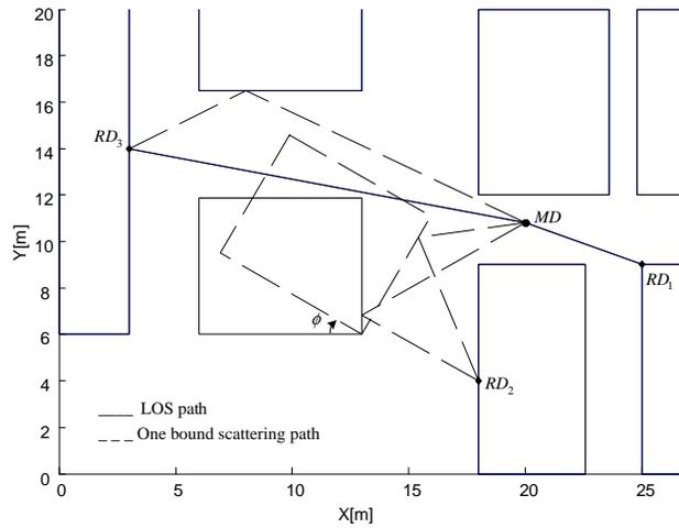
**Figure 11.** Ray tracing between the  $RDs$  and  $MD$  for different degrees of titled scatterer for distance standard deviation  $\sigma_d = 1$  m and AOA standard deviation  $\sigma_\alpha = 2^\circ$ .
