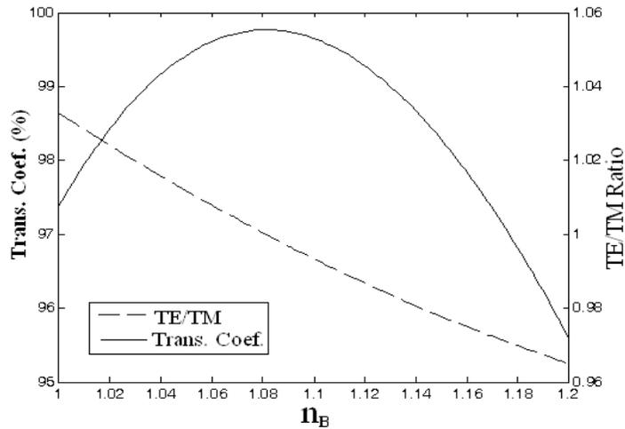
**Figure 4.** Transmission coefficients and TE/TM ratio of a PPCS.
