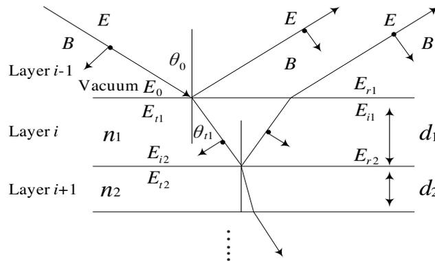
**Figure 3.** Reflection and transmission in a PPCS.
