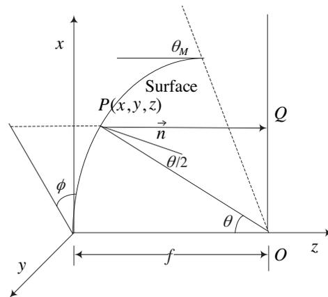
**Figure 2.** Ray tracing on the paraboloidal reflector.
