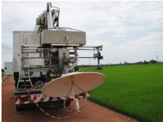
**Figure 4.** AAPS installed on the proposed scatterometer system.
