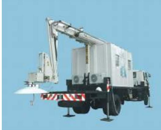
**Figure 3.** Antenna mounting in previous scatterometer system.
