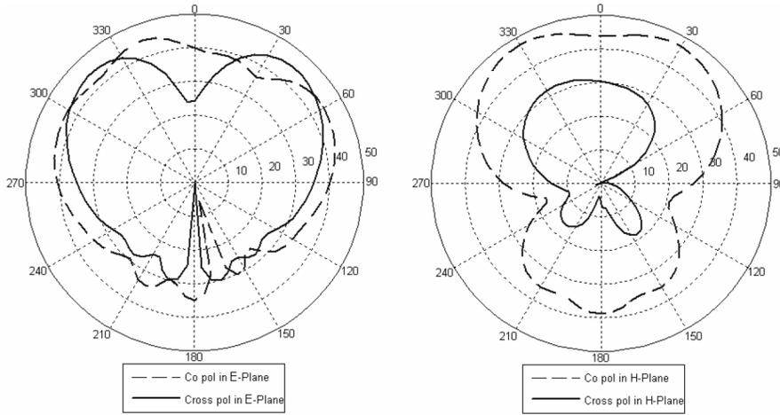
**Figure 13.** Measured co-pol and cross-pol radiation patterns at three frequencies of 7 GHz.
