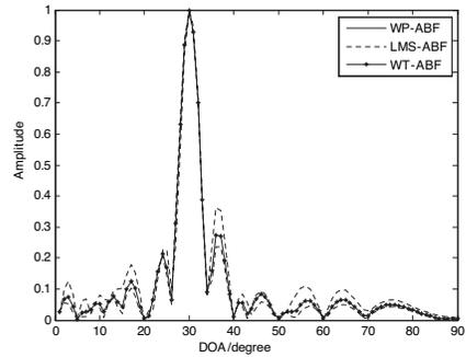
**Figure 7.** Beamforming performance comparison.
