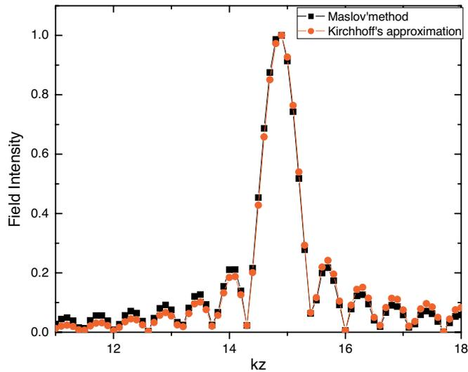
**Figure 2.** Comparison field Intensity at focal point of Wood lens Into uniaxial crystal by Maslov's method and Kirchhoff's approximation.
