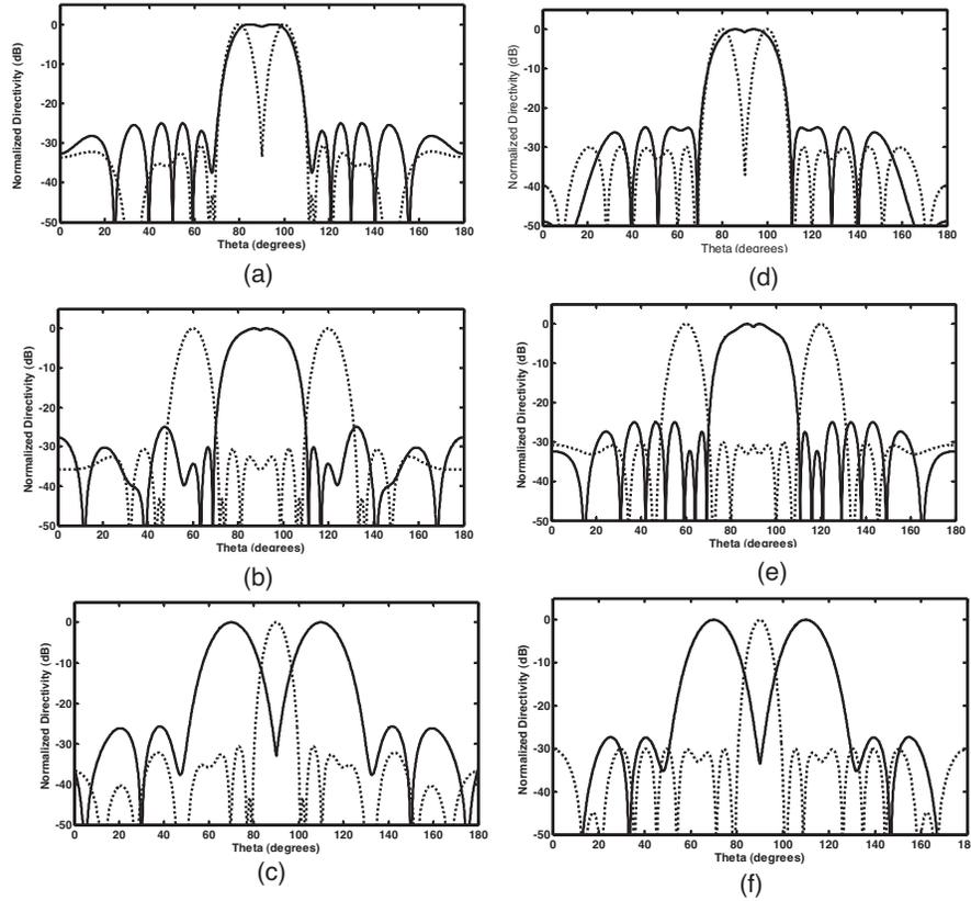
**Figure 4.** Scanning properties of optimised array patterns for element position perturbations of  $\pm 5\%$  (a) pencil beam  $10^\circ$  (b) pencil beam  $30^\circ$  (c) sector beam  $30^\circ$  and  $10\%$  (d) pencil beam  $10^\circ$  (e) pencil beam  $30^\circ$  (f) sector beam  $30^\circ$  and  $\pm 10\%$ .
