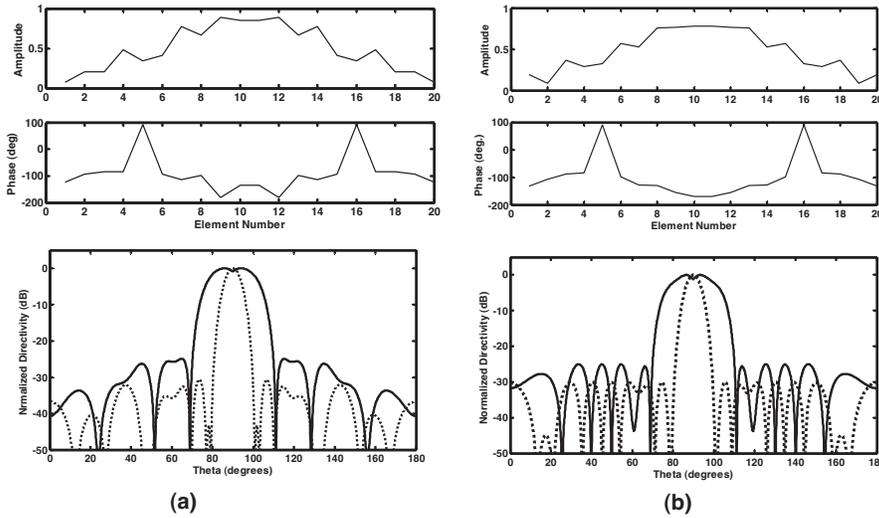
**Figure 3.** Dual beam optimised array patterns using element position perturbations of (a)  $\pm 5\%$  and (b)  $\pm 10\%$  for the corresponding excitation amplitudes-phase; ----- indicates the pencil beam and ——— indicates the fan shaped beam.
