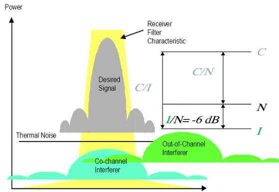
**Figure 2.** Types of interference and coexistence criterion.
