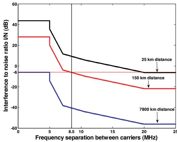
Figure 5. Interference from 10 MHz WiMAX into 7 MHz FWA.
