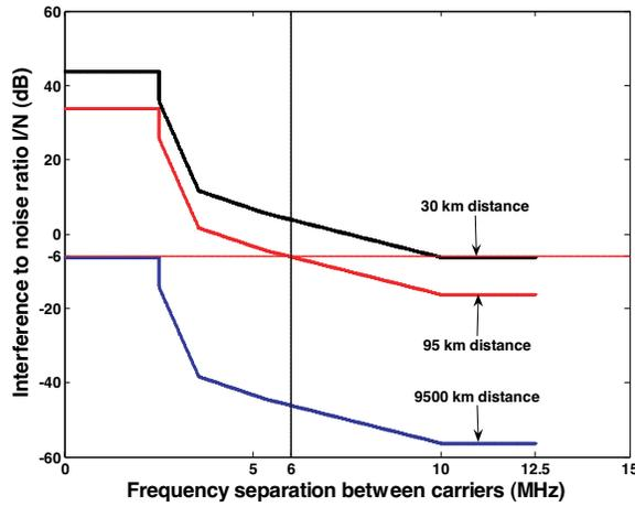
Figure 4. Interference from 5 MHz WiMAX into 7 MHz FWA.
