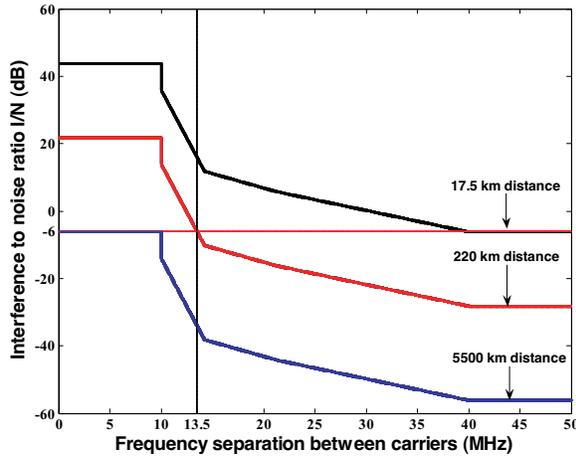
Figure 6. Interference from 20 MHz WiMAX into 7 MHz FWA.
