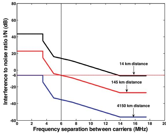
Figure 7. Interference from 7 MHz FWA into 5 MHz WiMAX.
