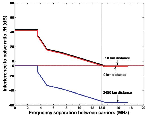
Figure 9. Interference from 7 MHz FWA into 20 MHz WiMAX.
