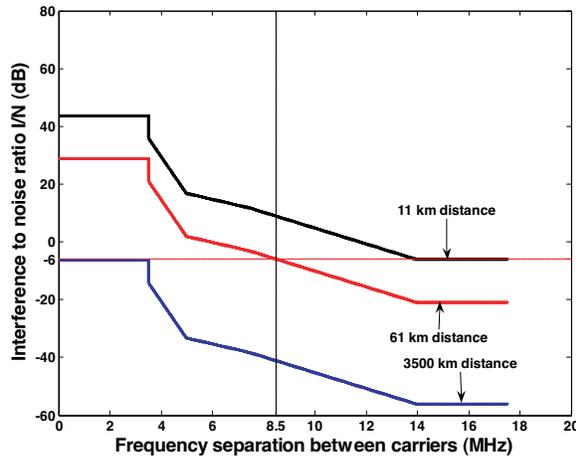
Figure 8. Interference from 7 MHz FWA into 10 MHz WiMAX.
