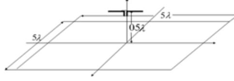
**Figure 6.** A dipole on a rectangular ground plane.
