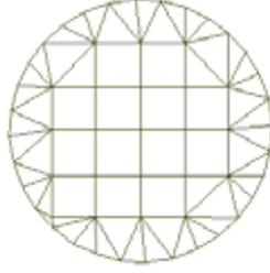
**Figure 3.** Mixed-face model of a circular surface.
