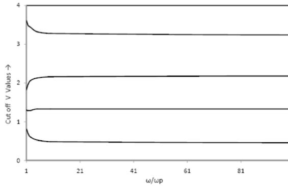
**Figure 5.** The variation of cutoff frequency  $V_c$  for different guided modes as a function of  $\frac{\omega}{\omega_p}$  for five layered Bragg fiber at  $d_2 = 0.25 \mu\text{m}$ .
