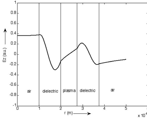
**Figure 6.** The E.M. field distribution of the proposed Bragg fiber mode with  $E_z$  component at  $\frac{\omega_p}{\omega} = 0.4$  fixed.
