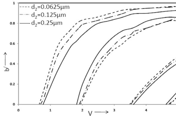
**Figure 4.** Dispersion characteristics curves of the proposed Bragg fiber for three cladding layers with three different values of  $d_2$  keeping  $\frac{\omega_p}{\omega} = 0.4$  fixed.
