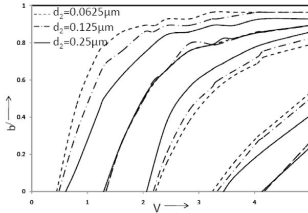
**Figure 3.** Dispersion characteristics curves of the proposed Bragg fiber for five cladding layers with three different values of  $d_2$  keeping  $\frac{\omega_p}{\omega} = 0.4$  fixed.
