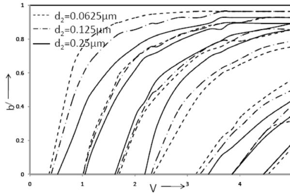
**Figure 2.** Dispersion characteristics curves of the proposed Bragg fiber for seven cladding layers with three different values of  $d_2$  keeping  $\frac{\omega_p}{\omega} = 0.4$  fixed.
