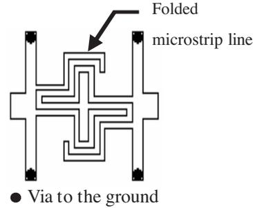
**Figure 2.** Top-view of the present CRLH TL unit.
