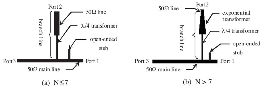
**Figure 7.** Top-view of the 3-port power dividers.
