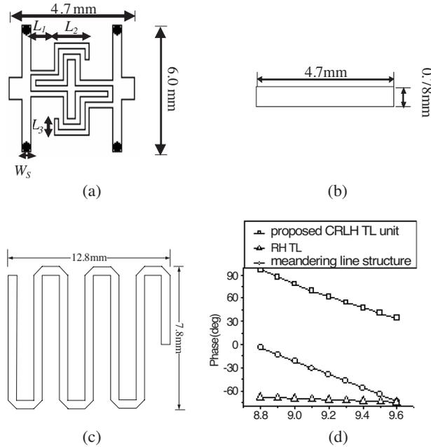
**Figure 8.** Comparison of phase delays of the three structures. (a) Top-view of the present CRLH TL unit,  $L_1 = 0.9$  mm,  $L_2 = 1.5$  mm,  $L_3 = 1$  mm,  $W_S = 0.4$  mm, the width of the folded lines 0.2 mm, the central spacing 0.33 mm, all the other spacings 0.2 mm; (b) Top-view of the traditional RH TL; (c) Meandering line structure; (d) Phase delay.
