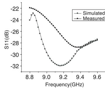
**Figure 10.**  $S_{11}$  of the series feed network.
