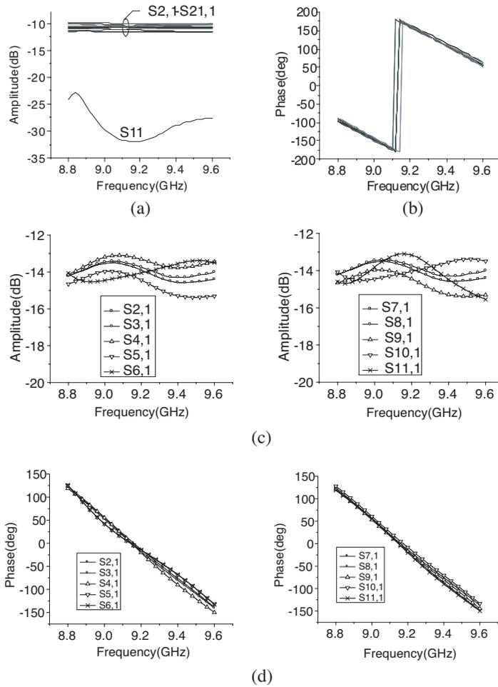
**Figure 11.** Simulated and measured results of the series feed network. (a) Simulated amplitude distributions; (b) Simulated phase distributions; (c) Measured amplitude distributions; (d) Measured phase distributions.
