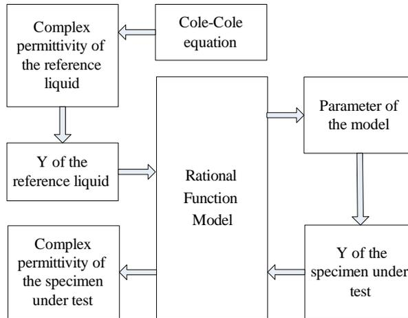
**Figure 1.** Principle of the permittivity measurement with rational function model.
