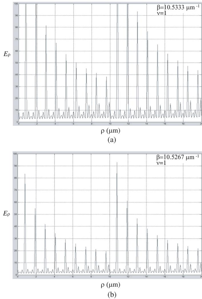
**Figure 3.** (a) Plot of the radial component of the electric field against the fiber radius corresponding to  $\rho_0 = 10 \mu\text{m}$ ,  $\psi = 90^\circ$  and  $\beta = 10.5333 \mu\text{m}^{-1}$ . (b) Plot of the radial component of the electric field against the fiber radius corresponding to  $\rho_0 = 10 \mu\text{m}$ ,  $\psi = 90^\circ$  and  $\beta = 10.5267 \mu\text{m}^{-1}$ .
