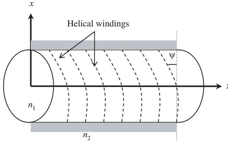
**Figure 1.** Schematic diagram of a helical clad fiber.
