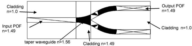
**Figure 10.** Acrylic-based  $1 \times 2$  POF coupler block layout for ray tracing.
