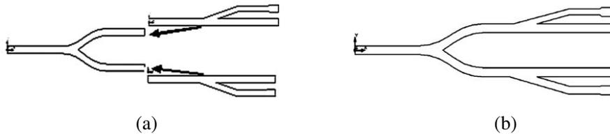
**Figure 3.** (a)  $1 \times 2$  Y-junction coupler before joining with two asymmetric  $1 \times 2$  couplers (b)  $1 \times 4$  coupler with asymmetric branches.
