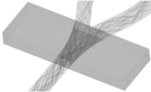
**Figure 8.** Close up view ray tracing of the metal-based hollow taper region.
