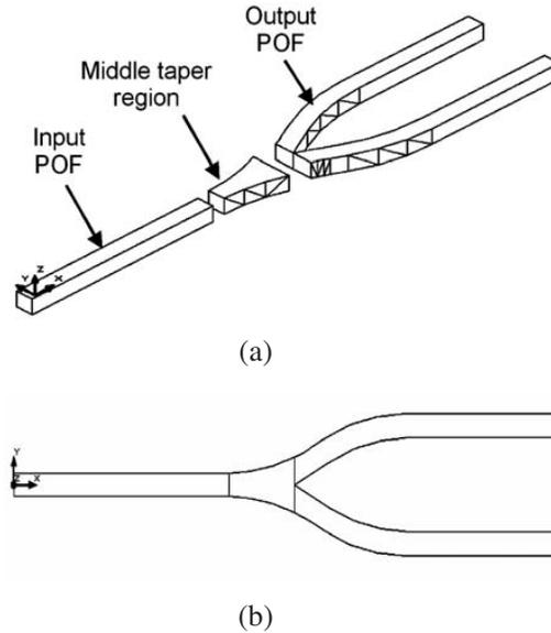
**Figure 6.** CAD design of the acrylic-based  $1 \times 2$  POF coupler. (a) Input POF, taper region, output POF, (b) POF coupler after combining.
