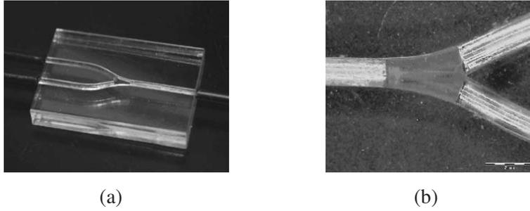
**Figure 15.** Fabricated acrylic-based  $1 \times 2$  POF coupler (a) assembled coupler with POF fibers (b) coupler showing the middle taper waveguide region and the input and output POF fibers.
