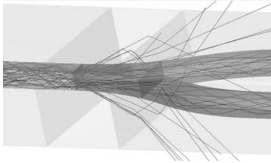
**Figure 12.** Close up view ray tracing of the acrylic-based taper region.
