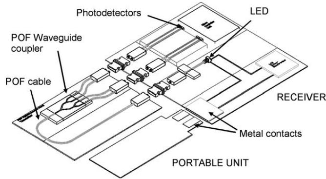
**Figure 2.** CAD diagram of the proposed optical access-card system.
