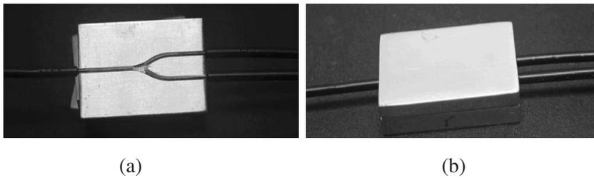
**Figure 14.** Fabricated metallic-based  $1 \times 2$  POF coupler devices (a) Y-branch coupler (b) coupler with top metal plate.
