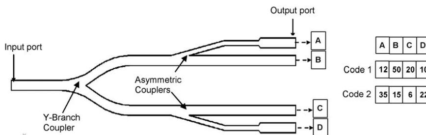
**Figure 1.** Code generating component for a  $1 \times 4$  waveguide coupler device (4-digit code).
