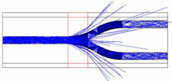
**Figure 11.** Ray tracing of the acrylic-based  $1 \times 2$  POF coupler.
