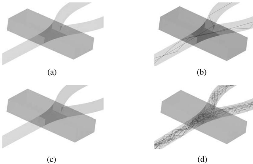
**Figure 9.** (a) No ray transmits out of (or refract out) of the hollow region (b) Rays that do not reflect on the inner surface of the middle taper region but pass through it (c) No scattering rays (d) Outgoing rays from the hollow taper region are all transmitted into the output branch POF fibers.
