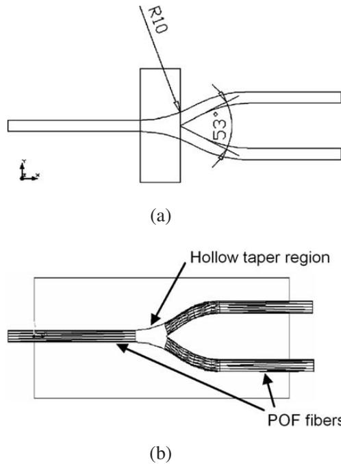
**Figure 4.** Metal-based  $1 \times 2$  POF coupler (a) 2D CAD layout (b) POF coupler layout with input and output POF fibers.
