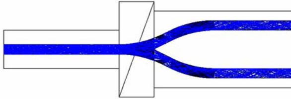
**Figure 7.** Ray tracing of the metal-based  $1 \times 2$  POF coupler with a middle hollow taper waveguide.
