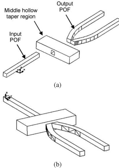
**Figure 5.** CAD design of the metal-based  $1 \times 2$  POF coupler. (a) Input POF, middle hollow taper and output POF, (b) POF coupler after combining.
