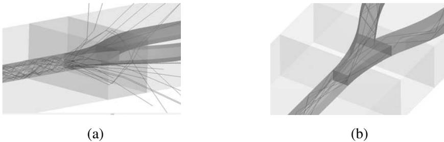
**Figure 13.** (a) Rays leak out or transmit out of the middle taper core region. (b) Rays that do not reflect on the inner surface of the middle taper region but pass through it.
