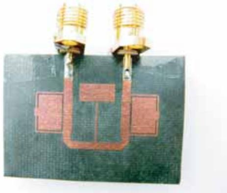
**Figure 7.** Fabricated ‘Butterfly’ via-less UWB microstrip filter.
