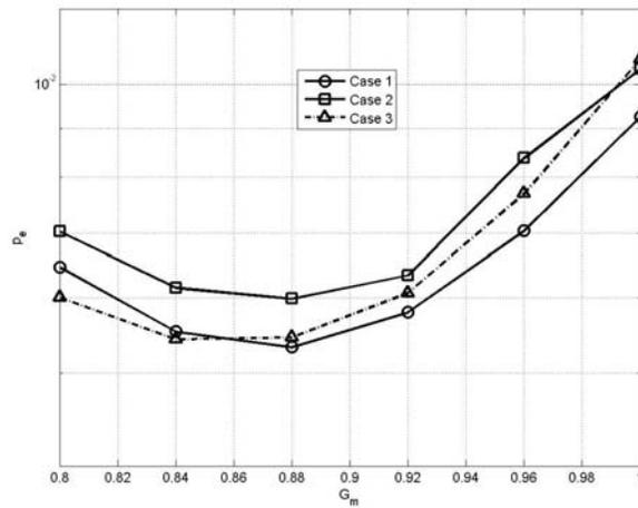
**Figure 9.** The error rate performance as to several values of  $G_m$  parameter. Case 1:  $p_e$  vs.  $G_m$  with  $W_m = 1.0[T_b]$  ( $SNR = 14$  dB). Case 2:  $p_e$  vs.  $G_m$  with  $W_m = 1.5[T_b]$  ( $SNR = 14$  dB). Case 3:  $p_e$  vs.  $G_m$  with  $W_m = 2.0[T_b]$  ( $SNR = 14$  dB).
