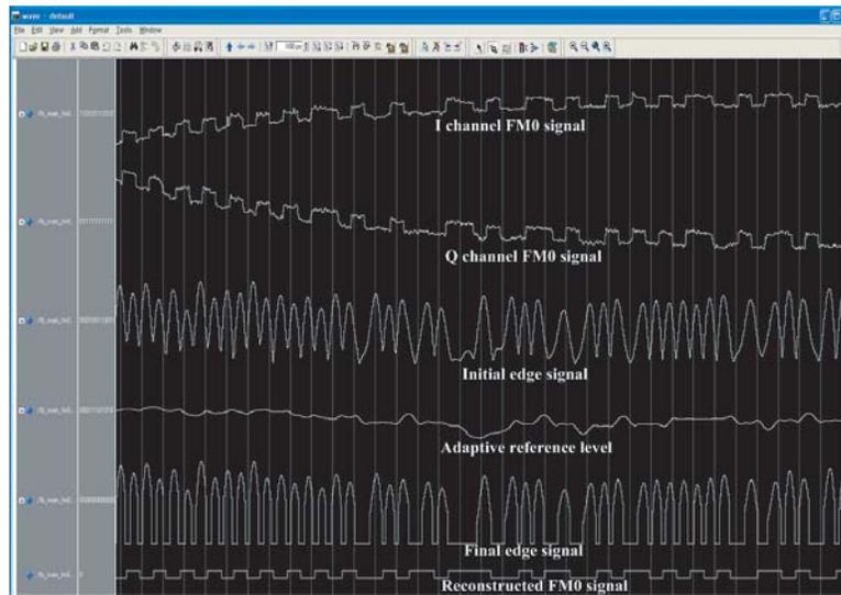
**Figure 11.** Timing simulation of the proposed demodulation structure.
