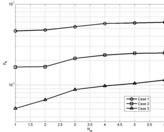
**Figure 7.** error rate performance as to several values of  $N_m$  parameter. Case 1:  $p_e$  vs.  $N_m$  ( $SNR = 13\text{dB}$ ). Case 2:  $p_e$  vs.  $N_m$  ( $SNR = 14\text{dB}$ ). Case 3:  $p_e$  vs.  $N_m$  ( $SNR = 15\text{dB}$ ).
