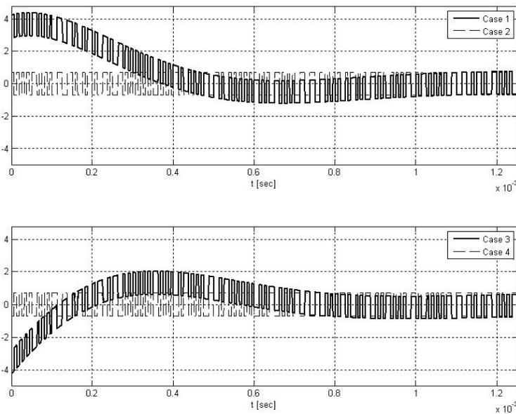
**Figure 2.** I-channel and Q-channel FM0 received signals distorted by DC-offset noise when the number of FM0 symbols is 100. Case 1 and Case 3 represent the I-channel and the Q-channel received signals with DC-offset noise. Case 2 and Case 4 represent the I-channel and the Q-channel received signals without DC-offset noise.
