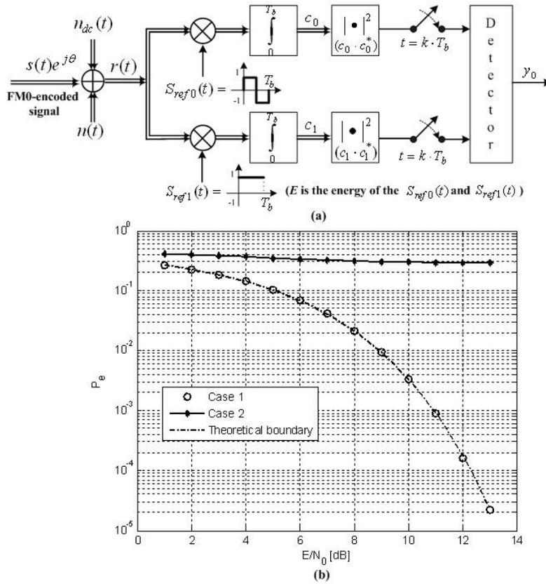
**Figure 3.** The error rate performance as to DC-offset noise for a traditional receiver with optimal detector. Case 1 denotes the  $p_e$  without DC-offset noise. Case 2 denotes the  $p_e$  with DC-offset noise.
