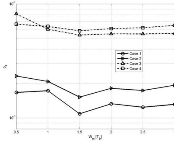
**Figure 8.** The error rate performance as to several values of  $W_m$  parameter. Case 1:  $p_e$  vs.  $W_m$  with  $G_m = 0.88$  ( $SNR = 16$  dB). Case 2:  $p_e$  vs.  $W_m$  with  $G_m = 0.92$  ( $SNR = 16$  dB). Case 3:  $p_e$  vs.  $W_m$  with  $G_m = 0.88$  ( $SNR = 14$  dB). Case 4:  $p_e$  vs.  $W_m$  with  $G_m = 0.92$  ( $SNR = 14$  dB).
