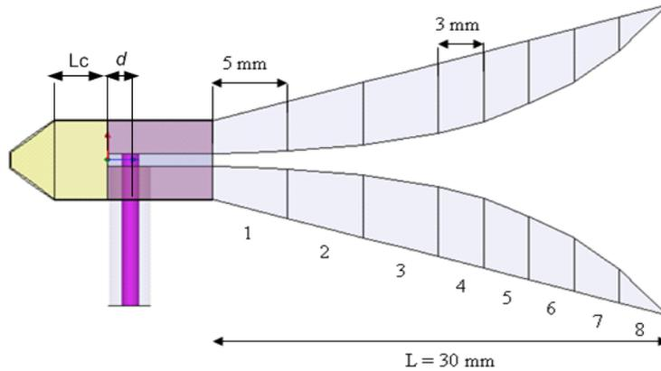
**Figure 6.** The proposed antenna made from eight smaller waveguides each of different height (cut view).
