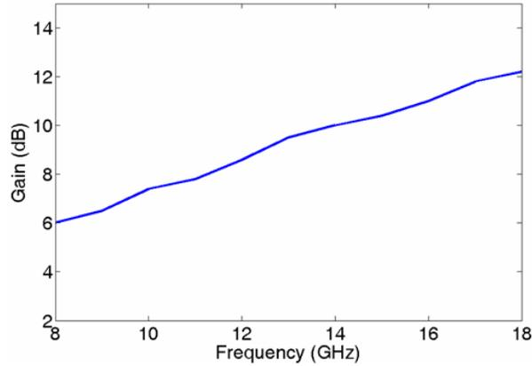
**Figure 11.** Gain versus frequency for the proposed antenna.
