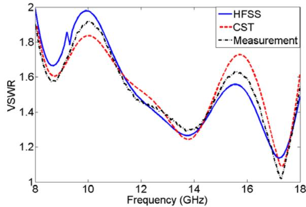
**Figure 8.** Simulated and measured VSWR of the designed antenna.
