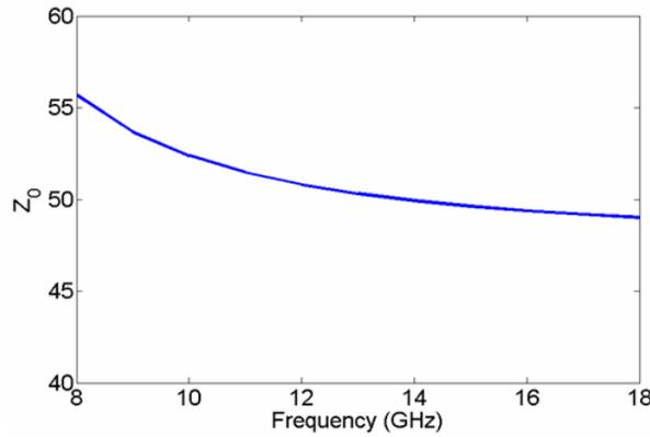
**Figure 4.** Characteristic impedance of the fundamental propagation mode (TE<sub>10</sub>) versus frequency.
