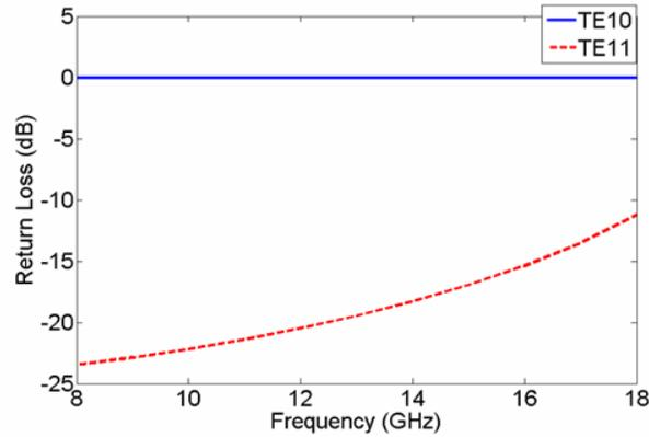
**Figure 3.**  $S_{12}$  parameter of the propagation mode (TE<sub>10</sub>) and non-propagation mode (TE<sub>11</sub>) versus frequency.
