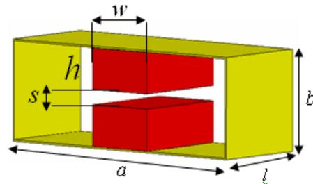
**Figure 2.** Two port double-ridged rectangular waveguide without coaxial probe.
