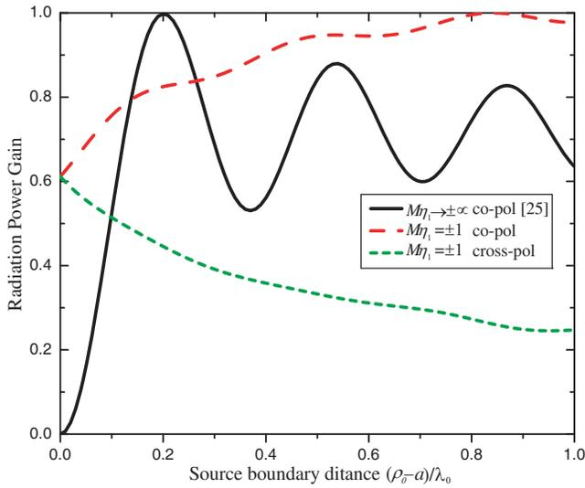
**Figure 4.** Radiation power gain of a PEMC circular cylinder as a function of distance of line source from the cylinder boundary when DNG coating layer is used i.e.,  $(\epsilon_r = -1.5, \mu_r = -1.5)$  when  $a = 1.25\lambda_0$ ,  $b = 3\lambda_0$ ,  $\rho_0 = 1.4\lambda_0$ .
