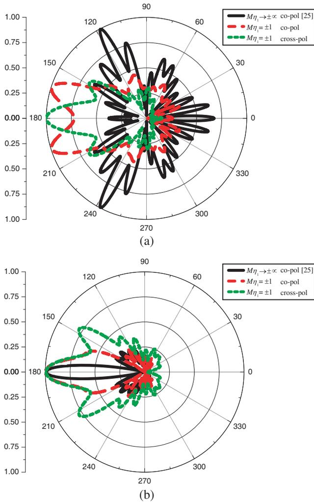
**Figure 2.** (a) Far-field radiation patterns of a PEMC circular cylinder coated by DPS layer ( $\epsilon_r = 1.5$ ,  $\mu_r = 1.5$ ) when  $a = 1.25\lambda_0$ ,  $b = 2.2\lambda_0$ ,  $\rho_0 = 2.3\lambda_0$ , (b) far-field radiation patterns of a PEMC circular cylinder coated by DNG layer ( $\epsilon_r = -1.5$ ,  $\mu_r = -1.5$ ) when  $a = 1.25\lambda_0$ ,  $b = 2.2\lambda_0$ ,  $\rho_0 = 2.3\lambda_0$ .
