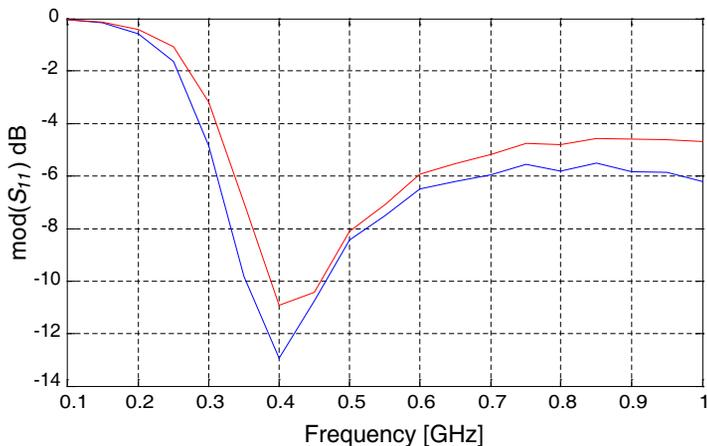
**Figure 14.** Comparison between the modulus of  $S_{11}$  scattering parameter of reference antenna (blue line) and reconfigurable antenna (red line) in the case of the relative dielectric permittivity of the investigated medium equal to 9.
