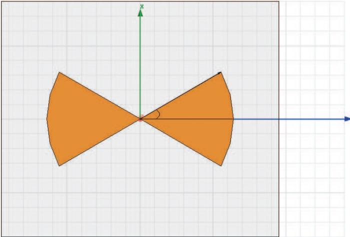
**Figure 1.** Reference bow-tie antenna: thickness  $36 \mu\text{m}$ , radius 64 mm and flared angle 30 degree, placed on substrate epoxy FR4 with extent  $20 \text{ cm} \times 20 \text{ cm} \times 3 \text{ mm}$ .
