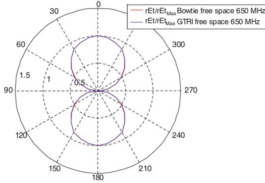
**Figure 8.** Comparison between the radiation patterns in the  $E$ -field at 650 MHz: reference antenna (red line) and reconfigurable antenna (blue line).
