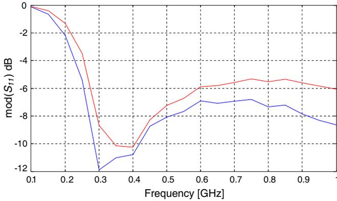
**Figure 15.** Comparison between the modulus of  $S_{11}$  scattering parameter of reference antenna (blue line) and reconfigurable antenna (red line) in the case of the relative dielectric permittivity of the investigated medium equal to 20.
