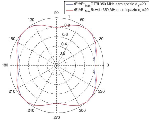
**Figure 17.** Comparison between the radiation patterns in the  $E$ -field at 350 MHz in the case of the relative dielectric permittivity equal to 20: reconfigurable antenna (blue line) and reference antenna (red line).
