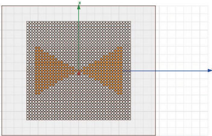
**Figure 2.** The reconfigurable antenna in the bow-tie geometry.
