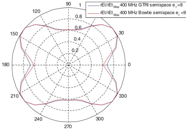
**Figure 16.** Comparison between the radiation patterns in the  $E$ -field at 400 MHz in the case of the relative dielectric permittivity equal to 9: reconfigurable antenna (blue line) and reference antenna (red line).
