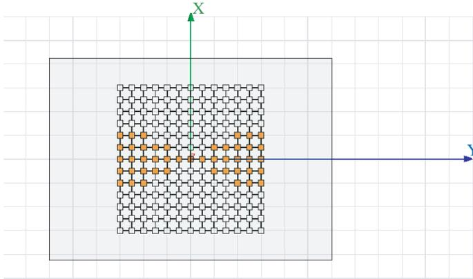
**Figure 10.** Reconfigurable bow-tie antenna with the  $5\text{ mm}\times 5\text{ mm}$  pads.
