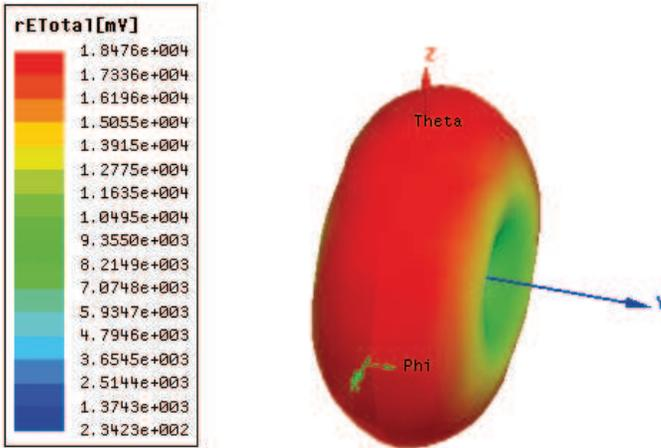
**Figure 9.** 3D-polar plot of the reconfigurable antenna in free space at 650 MHz.
