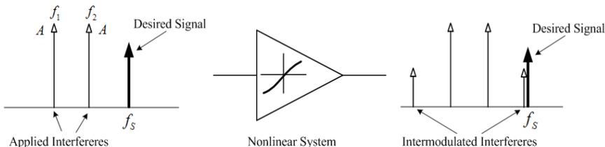
**Figure 1.** Intermodulation interference in a nonlinear system.
