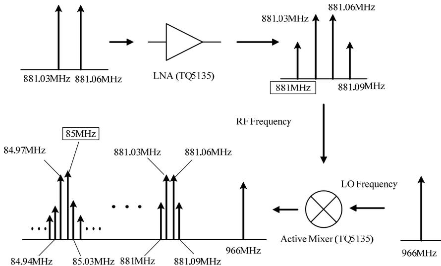
**Figure 2.** Frequency spectrum of the AMPS receiver IC TQ5135.
