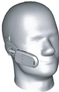
**Figure 1.** Complete model used for simulation including handset and SAM phantom head.
