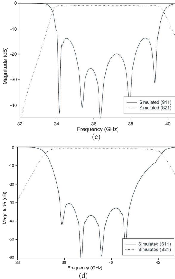
**Figure 4.** Simulated results of the designed three-line structure band-pass filters (a) filter one (26–30 GHz), (b) filter two (30–34 GHz), (c) filter three (34–38 GHz) and (d) filter four (38–40 GHz).
