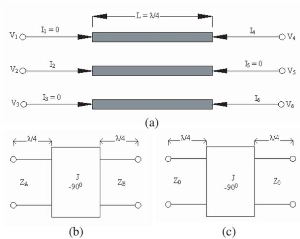
**Figure 3.** Equivalent circuit transform of the three-line structure (a) three-line structure as a six-port network, (b) equivalent admittance inverter and (c) further equivalent admittance inverter.
