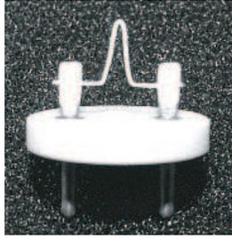
**Figure 12.** Photo of Thoria coated iridium filament.
