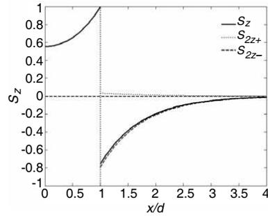
**Figure 7.** Energy flow at  $k_0d = 0.10$  for the surface wave mode with chirality and refractive index parameters  $\kappa_1 = 3.2, n_2 = 1.5, n_1 = 1.6$ .
