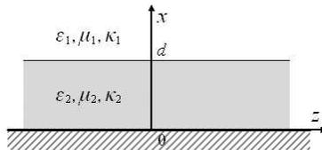
**Figure 1.** Geometry of the chiral negative refraction grounded slab waveguide.
