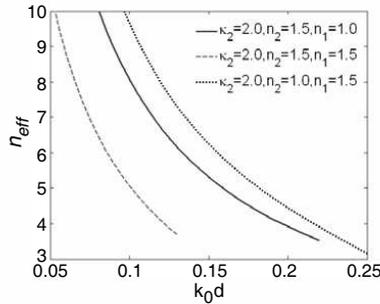
**Figure 2.** Dispersion curves of surface wave modes in the chiral negative refraction grounded slab waveguides.
