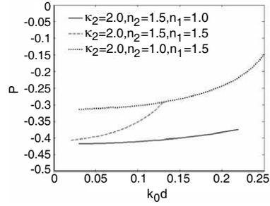
**Figure 5.** Normalized total power  $P$  versus normalized frequency  $k_0d$  for surface wave modes in the chiral negative refraction metamaterial grounded slab waveguides.
