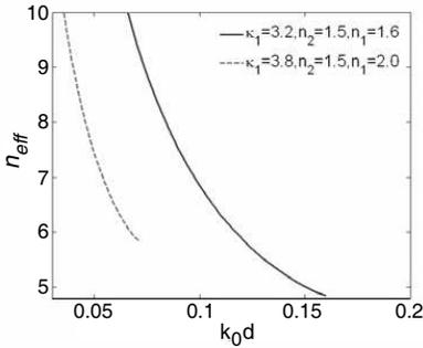
**Figure 6.** Dispersion curves of surface wave modes in the grounded slab with the chiral negative refraction cladding waveguides.
