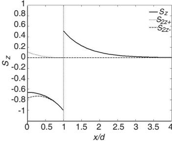
**Figure 4.** Energy flow at  $k_0d = 0.10$  for surface wave mode with refractive index parameters  $n_2 = 1.5, n_1 = 1.0$ .
