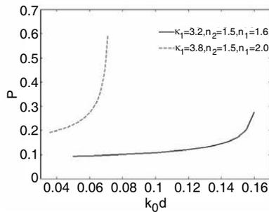
**Figure 8.** Normalized total power  $P$  versus normalized frequency  $k_0d$  for surface wave modes in the grounded slab with the chiral negative refraction cladding waveguides.
