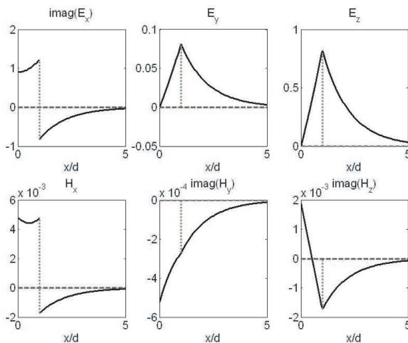
**Figure 3.** Amplitudes of electromagnetic field components at  $k_0d = 0.10$  for surface wave mode with refractive index parameters  $n_2 = 1.5, n_1 = 1.0$ .
