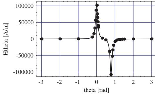
**Figure 6.** Representation of the azimuthal component  $H_\theta$  ( $r = 0.024$ ,  $\theta$ ,  $z = 0.002$ ) versus the angular displacement  $\theta$  with the following dimensions:  $r_1 = 0.025$  m,  $r_2 = 0.028$  m,  $h = z_2 - z_1 = 0.003$  m,  $J = 1$  T,  $r = 0.024$  m,  $\theta_2 - \theta_1 = \frac{\pi}{4}$  rad; (thick line = this work), (Points = Furlani's work [1]).
