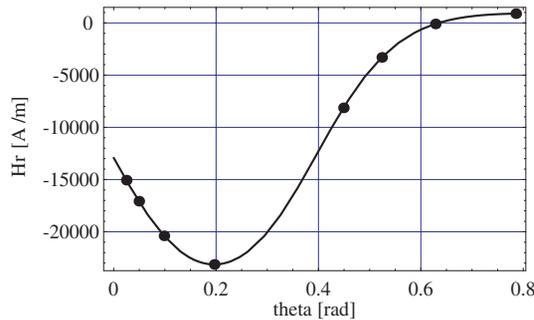
**Figure 5.** Representation of the radial component  $H_r$  ( $r = 0.02$  m,  $\theta, z = 0.0035$  m) versus the angular displacement  $\theta$  with the following dimensions:  $r_1 = 0.025$  m,  $r_2 = 0.028$  m,  $h = z_2 - z_1 = 0.003$  m,  $J = 1$  T,  $r = 0.02$  m; (thick line = this work), (Points = Furlani's work [1]).
