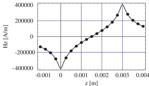
**Figure 3.** Representation of the axial component  $H_z(r = 0.0249$  m,  $z$ ) versus the axial displacement  $z$  with the following values:  $r_1 = 0.025$  m,  $r_2 = 0.028$  m,  $h = z_2 - z_1 = 0.003$  m,  $J = 1$  T; (thick line = amperian current model), (points = coulombian model).
