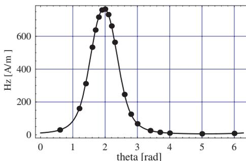
**Figure 7.** Representation of the axial component  $H_z$  ( $r = 0.015$ ,  $\theta$ ,  $z = 0.002$  m) versus the angular displacement  $\theta$  with the following dimensions:  $r_1 = 0.025$  m,  $r_2 = 0.028$  m,  $h = z_2 - z_1 = 0.003$  m,  $J = 1$  T,  $r = 0.015$  m,  $\theta_2 - \theta_1 = \frac{\pi}{4}$ ; (thick line = this work), (Points = Furlani's work [1]).
