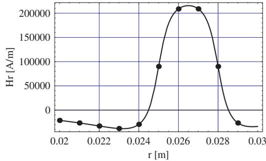
**Figure 2.** Representation of the radial component  $H_r(r, z = 0.0035)$  versus the radial displacement  $r$  with the following values:  $r_1 = 0.025$  m,  $r_2 = 0.028$  m,  $h = z_2 - z_1 = 0.003$  m,  $J = 1$  T; (thick line = amperian current model), (points = coulombian model).
