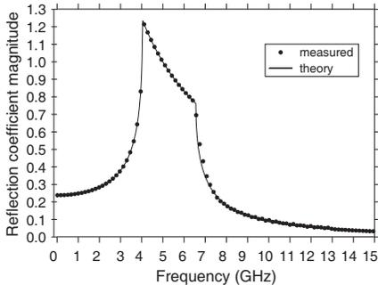
**Figure 4.** Magnitude of measured reduced interfacial reflection coefficient  $\tilde{\Gamma}$  compared to the theoretical value computed using  $\epsilon_r = 2.64$ . Below cutoff, the measured data is synthesized from the extracted value of  $\epsilon_r$ .
