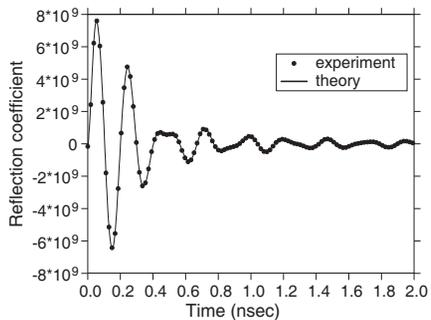
**Figure 7.** Time-domain reduced interfacial reflection coefficient obtained from an inverse FFT of the measured  $\Gamma$ , compared to that obtained using the time-domain formula with  $\epsilon_r = 2.64$ .
