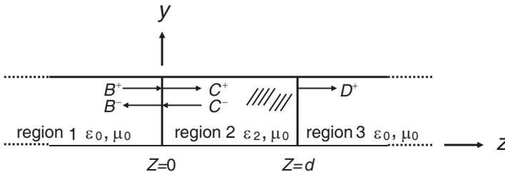
**Figure 1.** Side view of a rectangular waveguide loaded with a perfect dielectric material.
