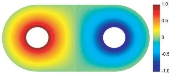
**Figure 3.** Port potential distribution for via-pair in shared antipad.
