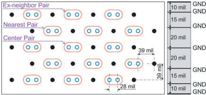
**Figure 4.** Via layout top view (left) and stack information on vertical cross-section (right).
