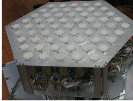
**Figure 2.** Photograph of SHA and RF front ends.
