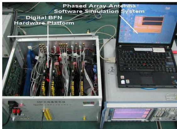
**Figure 8.** Photograph of semi-physical simulation platform (including digital BFN hardware platform).
