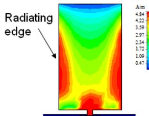
**Figure 1.** Current flow on a rectangular planar monopole.
