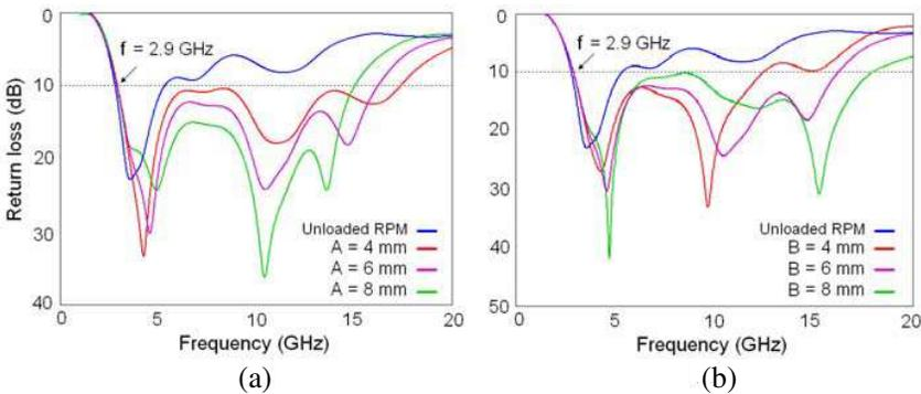
**Figure 4.** Return loss of RPM loaded with a pair of cylindrical plates with (a)  $B = 12$  mm, and different  $A$ , (b)  $A = 6$  mm and various  $B$ .
