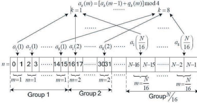
**Figure 3.** The structure of multi-beam OFDM symbol.
