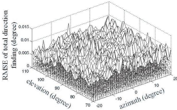
**Figure 10.** The total RMSE of direction finding in different directions.
