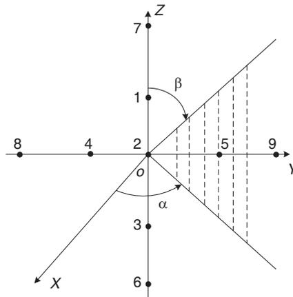
**Figure 1.** The coordinate system and the geometry of the sparse antenna array with nine elements, where  $D_g$ ,  $g = 1, 2, \dots, 9$  denote the spacing between  $g$ th element and the coordinate center,  $D_1 = D_4 = 2\lambda$ ,  $D_3 = D_5 = \frac{5}{2}\lambda$ ,  $D_2 = 0$ ,  $D_6 = D_7 = D_8 = D_9 = \frac{9}{2}\lambda$ ,  $\lambda$  is a wavelength,  $\alpha$  and  $\beta$  denote an azimuth angle and an elevation angle, respectively.
