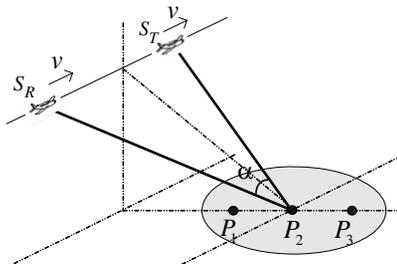
**Figure 5.** The illumination geometry for simulation Tandem configuration.
