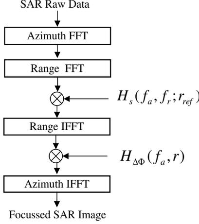
**Figure 3.** Flow diagram for the ETF algorithm.
