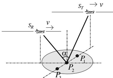
**Figure 8.** Illumination geometry for simulation forward-looking configuration.
