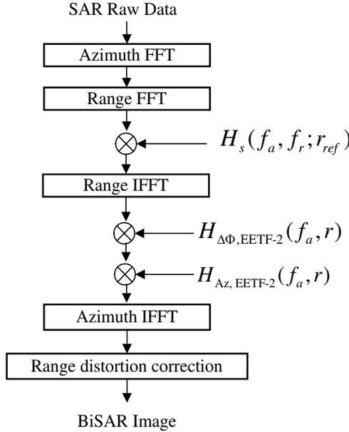
**Figure 4.** Flow diagram for the BiSAR EETF-2 algorithm.
