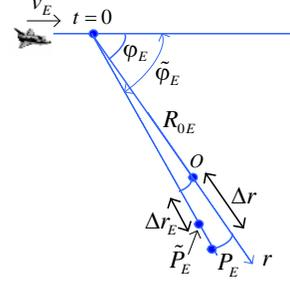
**Figure 2.** Imaging geometry of equivalent monostatic SAR.
